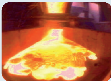
Corium flow experiment for the mastery of accident situations
