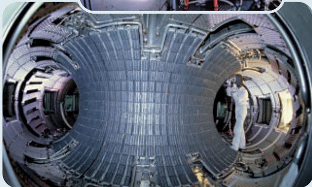
Toroidal chamber of the TORE SUPRA in which the plasma circulates during tests
