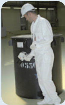
Radiological control on a low-level waste package
