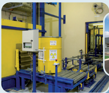
ROTONDE: the sorting and dispatching of low-level and very low-level waste packages
