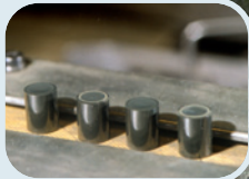
Nuclear fuel pellets currently used (mixed uranium and plutonium oxides)
