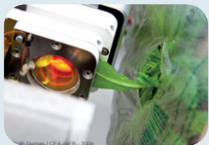
Measurement of gaseous exchanges on an Arabidopsis leaf
