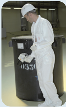
Radiological control on a low-level waste package
