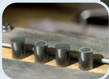
Nuclear fuel pellets currently used (mixed uranium and plutonium oxides)
